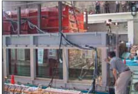
of the steel side walls minimized the effects of friction between the steel and the soils during the shaking.
